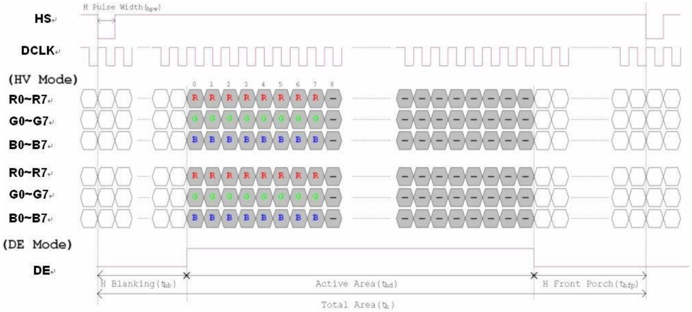
Figure 3. 1 Horizontal input timing diagram.
