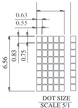
The non-specified tolerance of dimension is +0.3mm.
