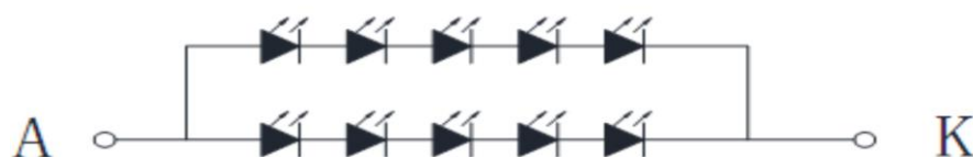
Backlight Circuit diagram (LED 5 \times 2 = 10 )
