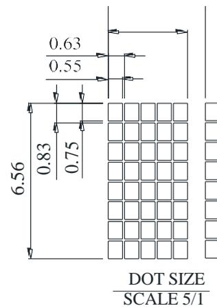
The non-specified tolerance of dimension is +0.3mm.
